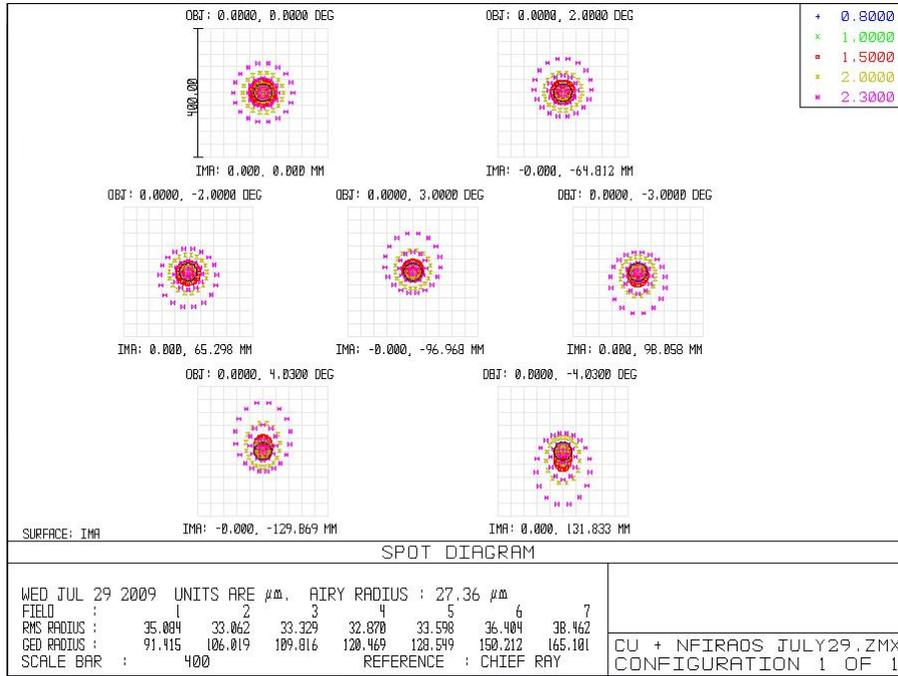
Figure 5. Spot diagrams of the combined optical design of NSCU and NFIRAOS at the NFIRAOS image plane. The wavelength coverage and fields are the same as Figure 4.
