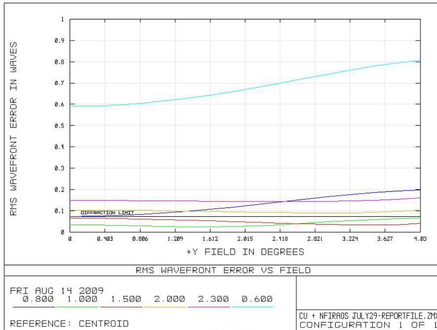
Figure 6. RMS wavefront error distribution along the off-axis fields at the NFIRAOS image plane of the combined optical design of NSCU and NFIRAOS for 0.8, 1.0, 1.5, 2.0, 2.3, and 0.6 microns.
