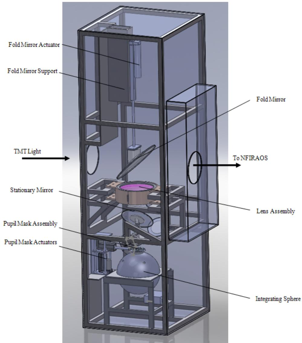
Figure 9. Opto-mechanical assembly of NSCU.
