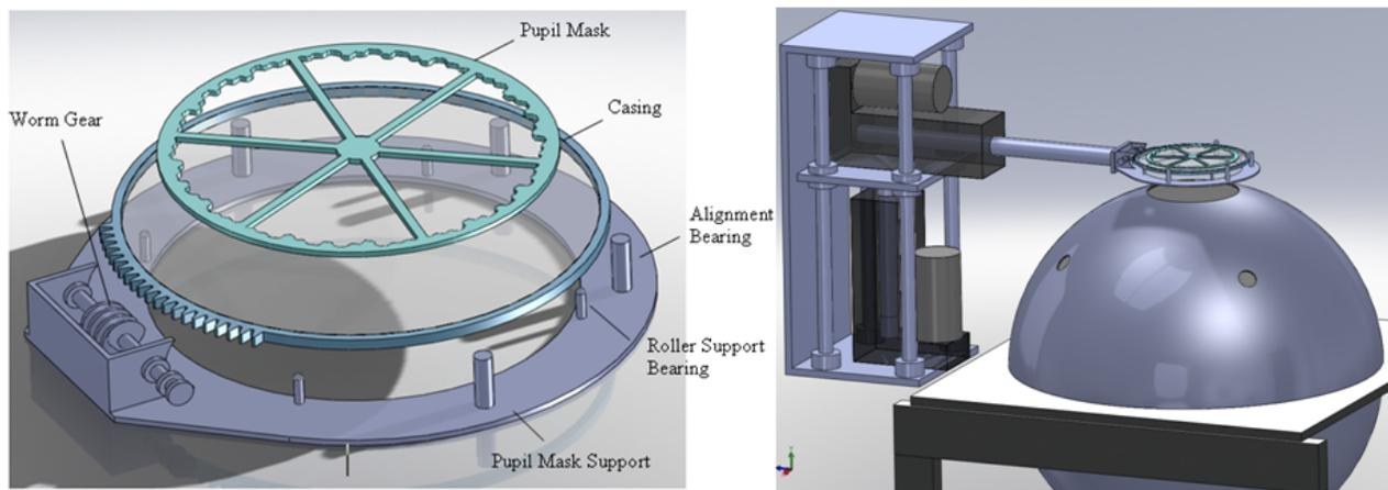
Figure 7. (Left panel) The mechanical assembly of the pupil-mask system of NSCU with a rotatable pupil mask at the top. (Right panel) The location of the pupil-mask system just outside of the integrating sphere. Note that it is retractable.
