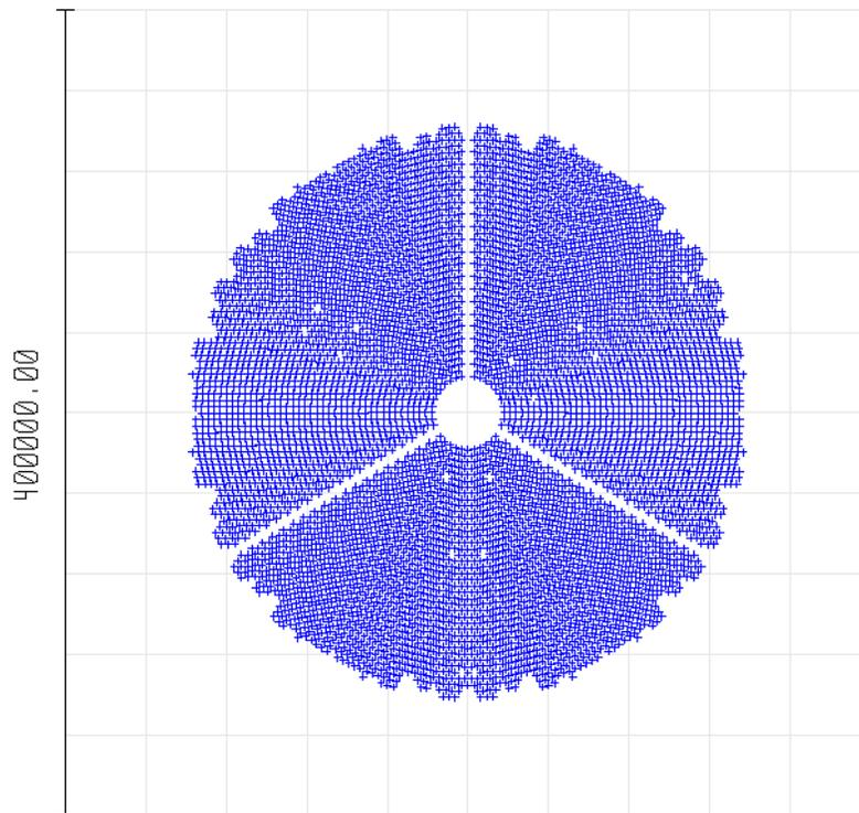
Figure 8. Pupil simulation spot diagram on DM0. The number in the left is in the unit of  $\mu\text{m}$ .
