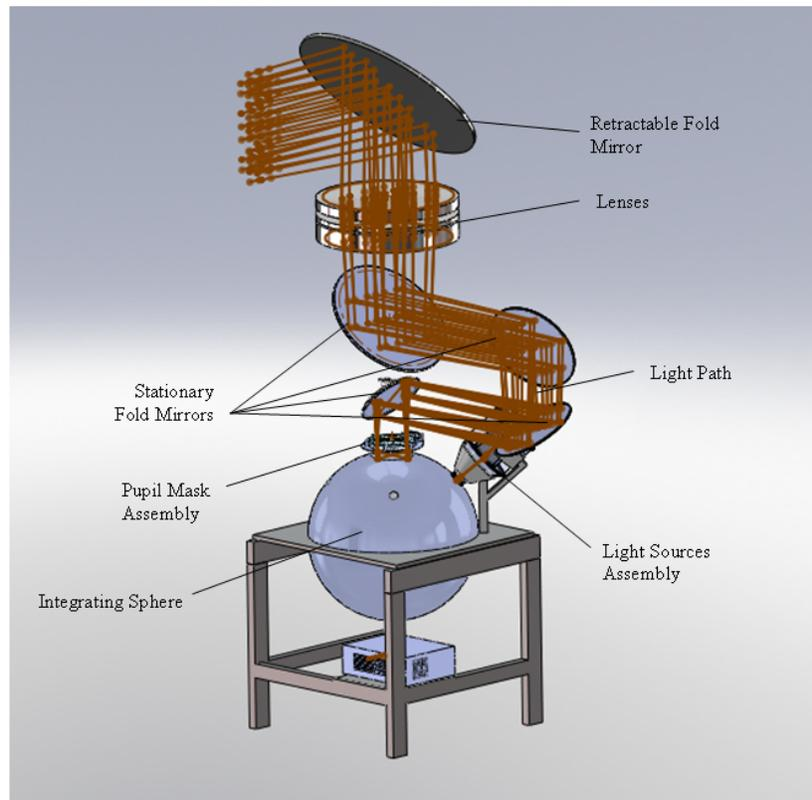
Figure 2. Optical path inside NSCU from the integrating sphere to the retractable fold mirror.
