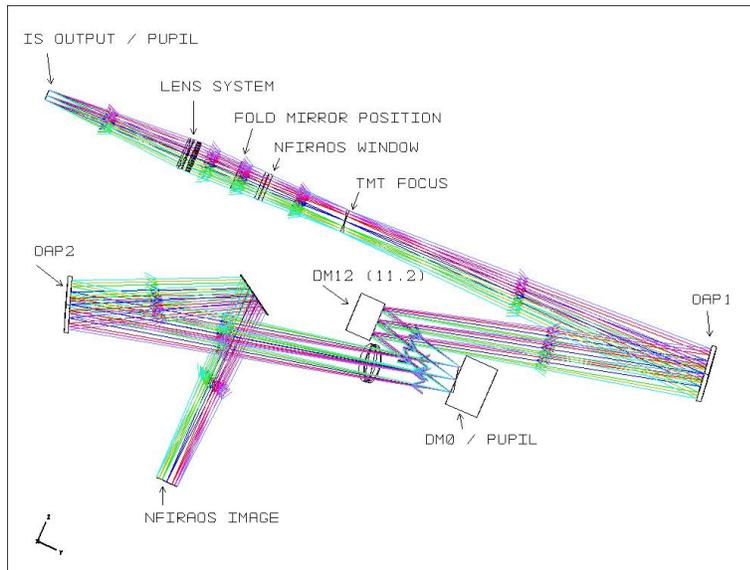
Figure 3. Ray-tracing layout of the combined NSCU and NFIRAOS optical system.
