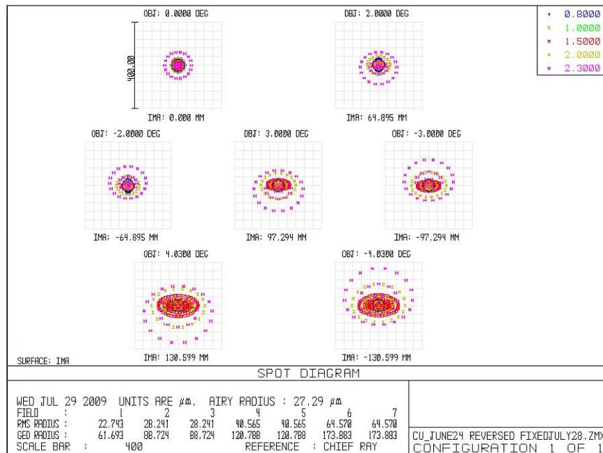
Figure 4. Spot diagrams of the stand-alone NSCU optical design at the TMT focal plane. The wavelength range is 0.8–2.4 micron and 8 different fields are shown from on-axis to 4-degree off-axis fields.
