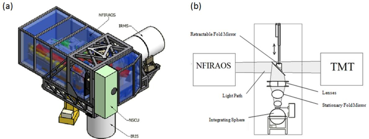
Figure 1. (a) The NSCU envelope location in front of NFIRAOS. (b) Basic configuration of the optical components inside NSCU.
