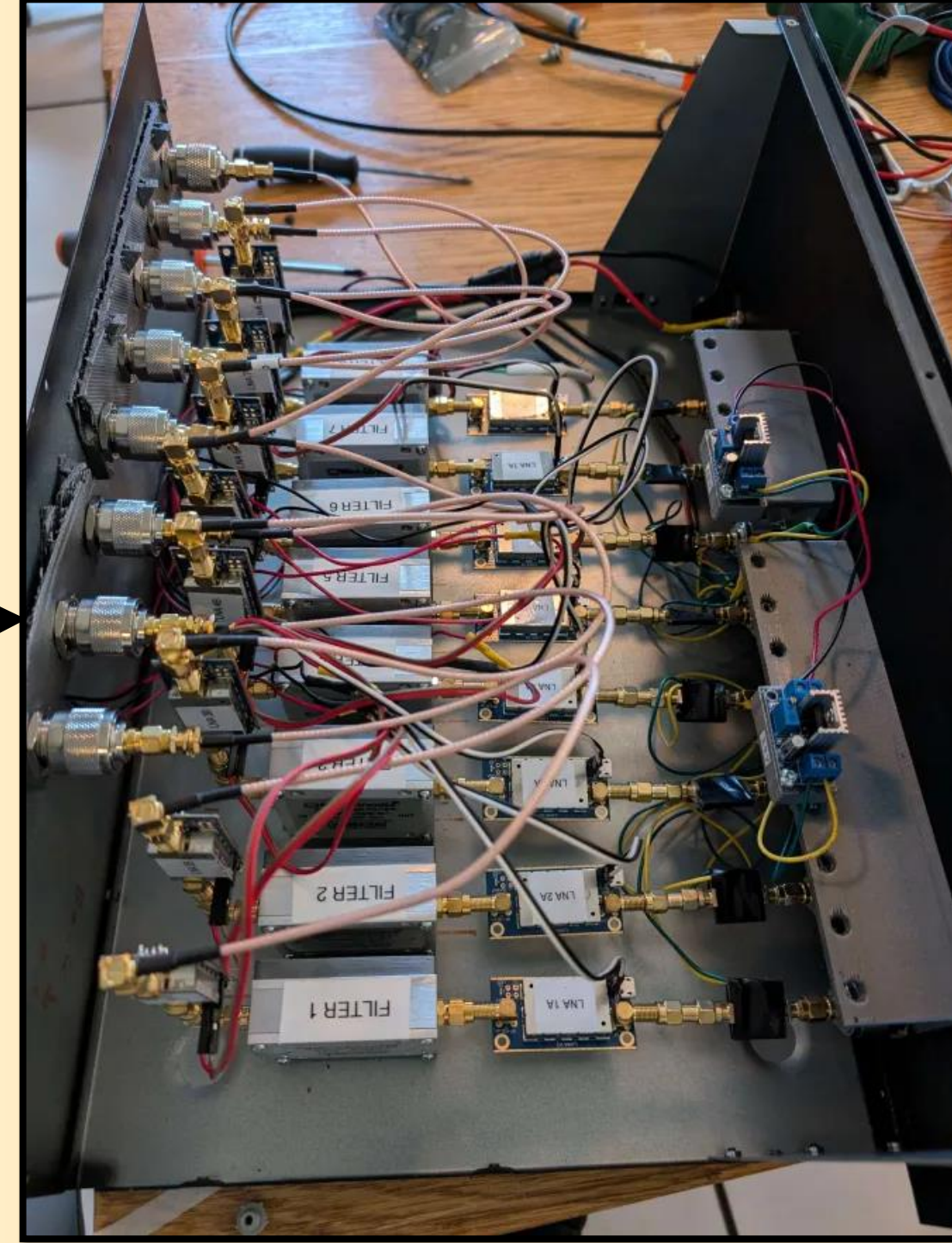
Amplifiers , 400-800 MHz bandpass filters , bias-tees , equalizers and voltage regulators for analog signal processing of AC voltages.
