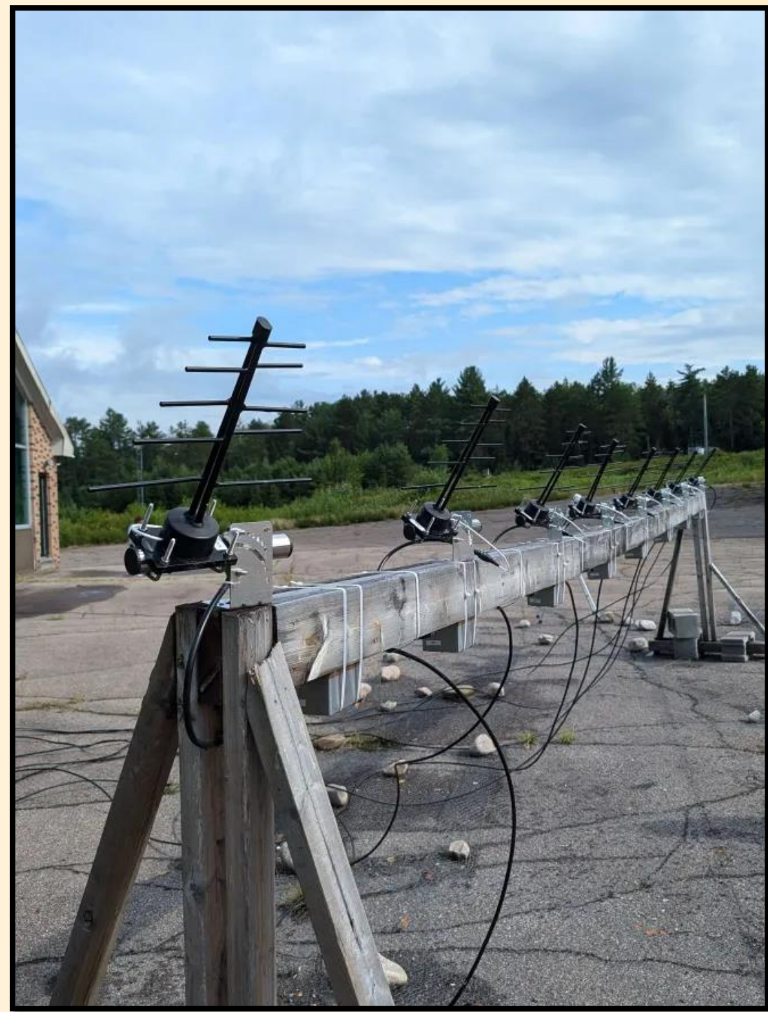
Log-periodic dipole array of 8 antennas at Algonquin Radio Observatory , 28 cross-correlations and 8 autocorrelations .
