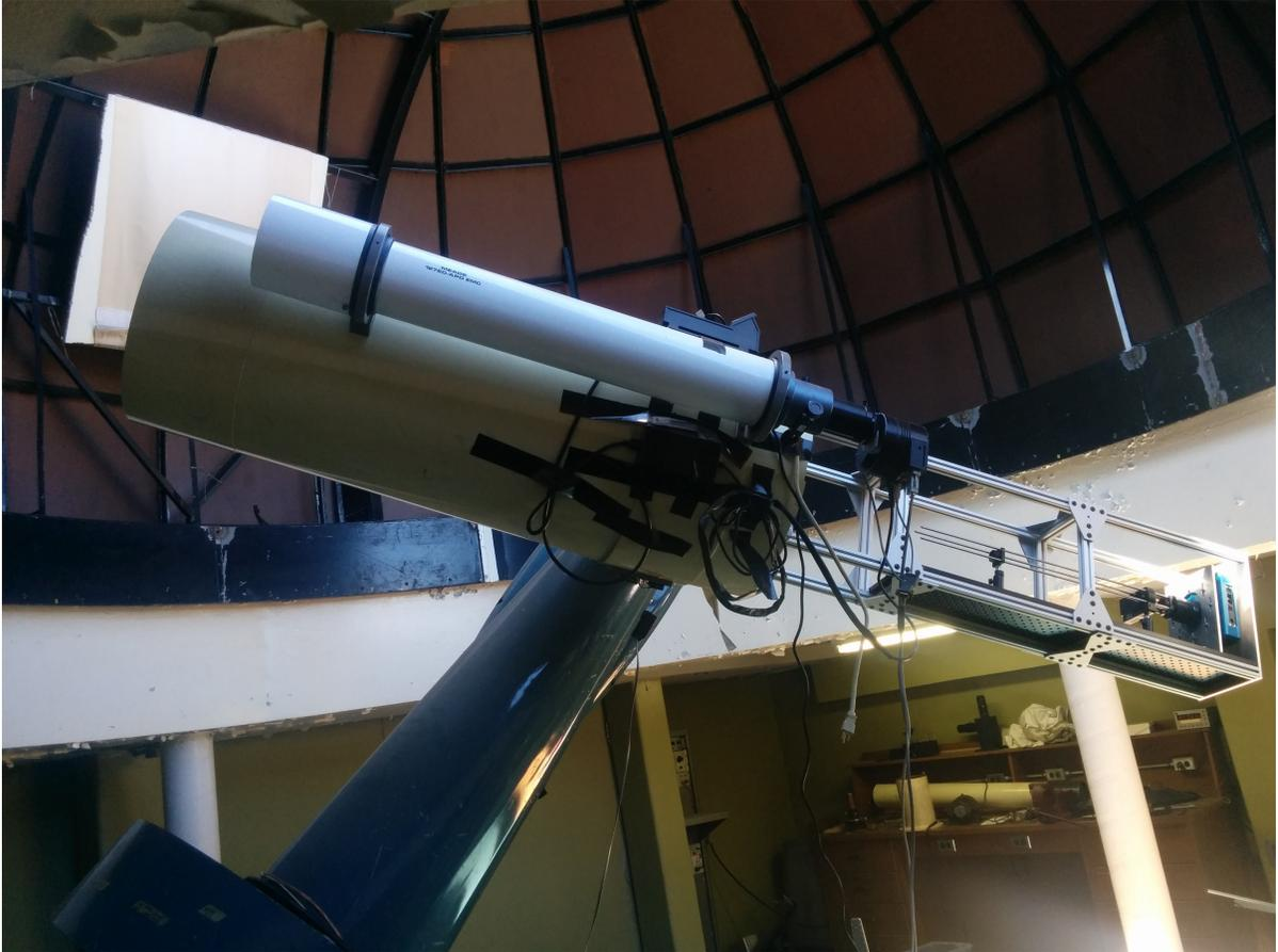
Figure 6.3: A photo of the PSP mounted on the 16-inch UofT telescope.
