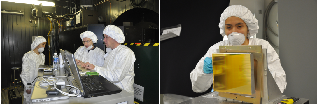
Figure 3.18 Left: OSIRIS team at the Nasmyth platform of Keck-I. The black dewar in the back is the Keck-I AO bench, and the green dewar on the right is the OSIRIS cooling enclosure. Right: Grating alignment with respect to the mounting plate in the lab at the Keck Observatory summit.
