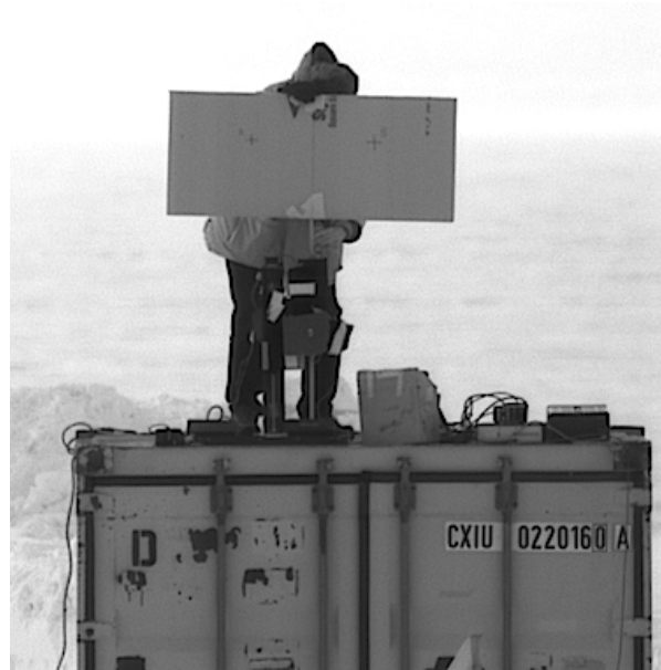
Figure 2.9: Setup for aligning the star cameras with the submillimeter beam. A piece of foam with two “+” markings is held a known distance above the submillimeter source being used for detector beam mapping.
