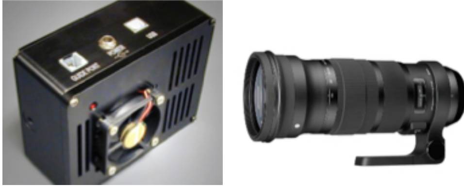
Figure 3.10: SBIG CCD camera (left) and Sigma lens (right) used in SPIDER star cameras.
