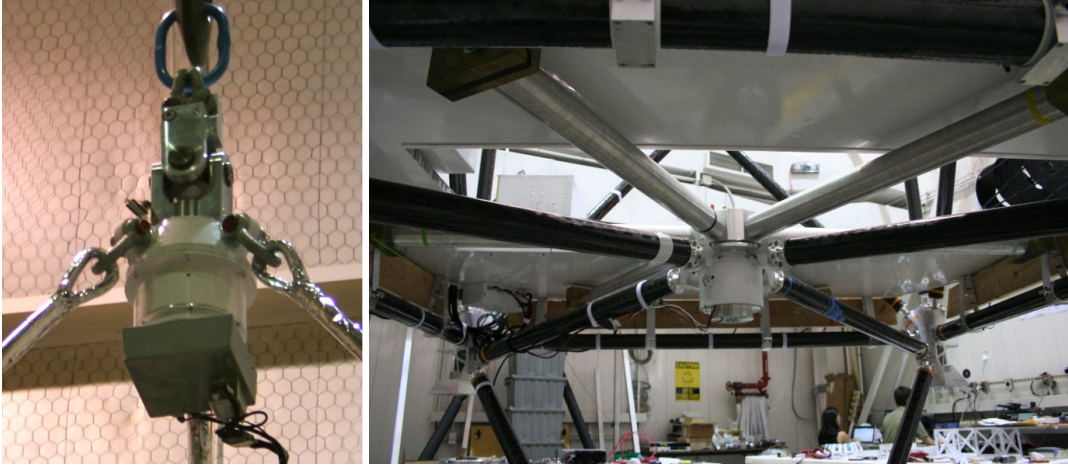
Figure 3.4: SPIDER azimuth motors. Left: Pivot; Right: Reaction wheel.
