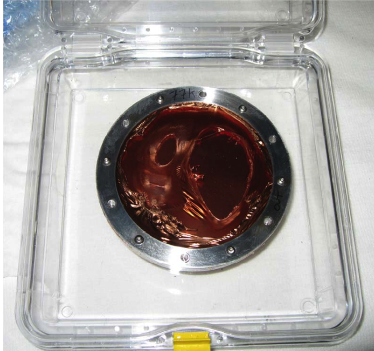
Figure 3.5: Picture of the first infrared blocking filter in the filter stack mounted just behind the cryostat window. This filter was first flown in 2010 (previous BLAST flights used a thicker filter) and was found to have been damaged after telescope recovery. The likely cause of the damage was sunlight incident on the filter while under vacuum.
