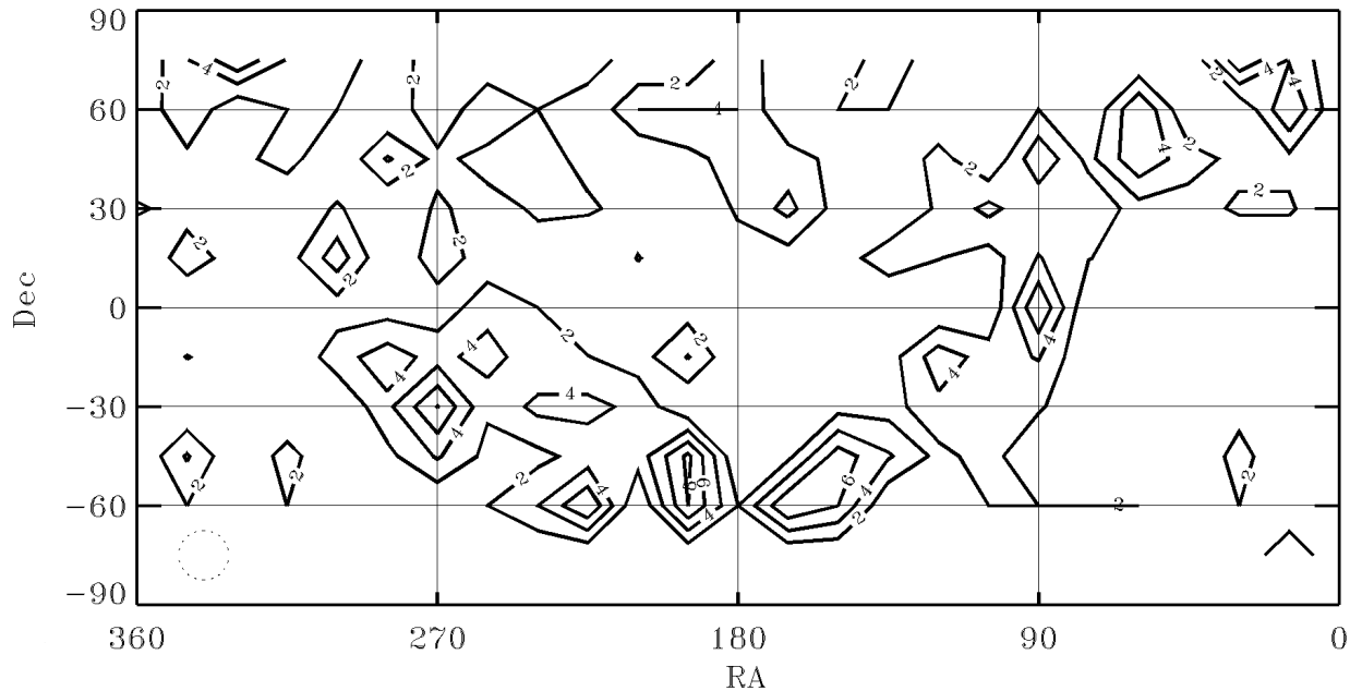
Fig.7. The sky density of stars to +3.5 apparent magnitude calculated for 15x15 degree fields. The contours are at intervals of 2, 4, 6, and 8 stars per field. The goals of the minimum mission can be accomplished in areas with star densities >2 per field. An extension in depth by one magnitude will increase stellar densities per 15x15 degree field by approximately 4 times; the same gain can be achieved by increasing the field size to 30x30 degrees.
