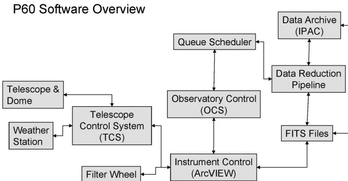
FIG. 5.—P60 software overview. Arrows indicate direct channels of communication. The modular design was chosen to ensure both stability and ease of upgrade/repair.
