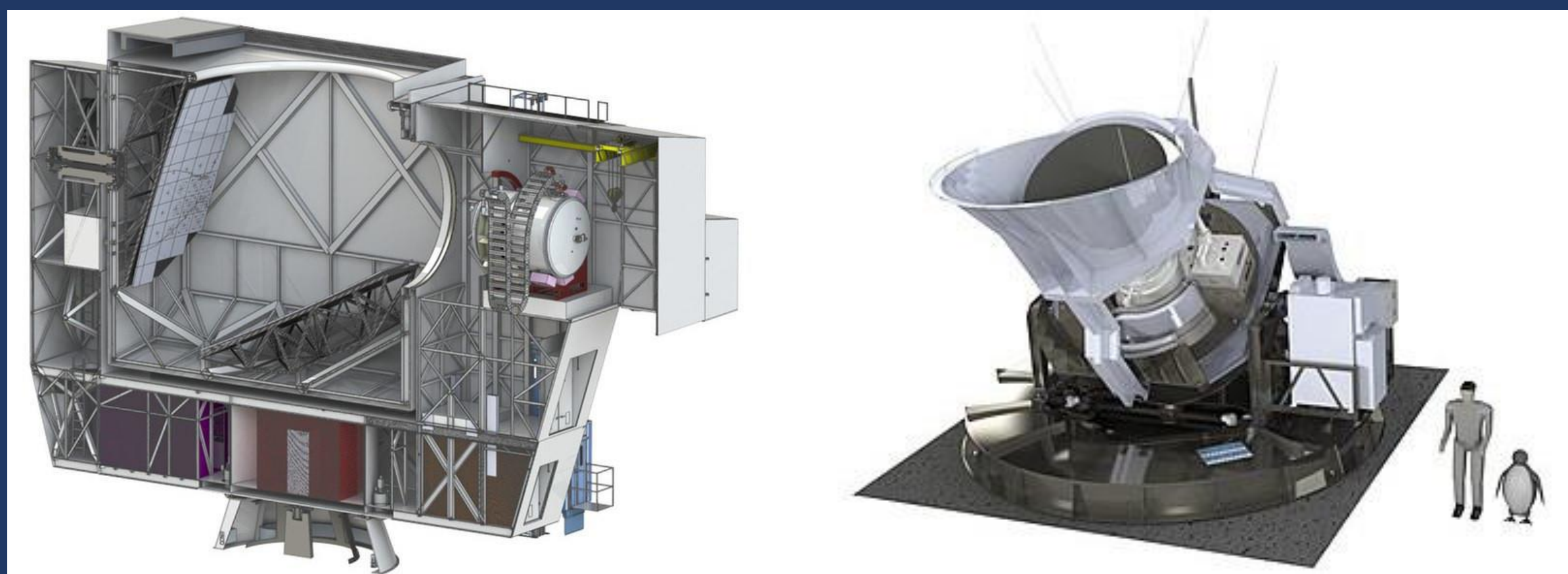
The design of the large (left) and small (right) aperture telescopes for SO. Human and penguin for scale. Figures taken from [2] and [3].
