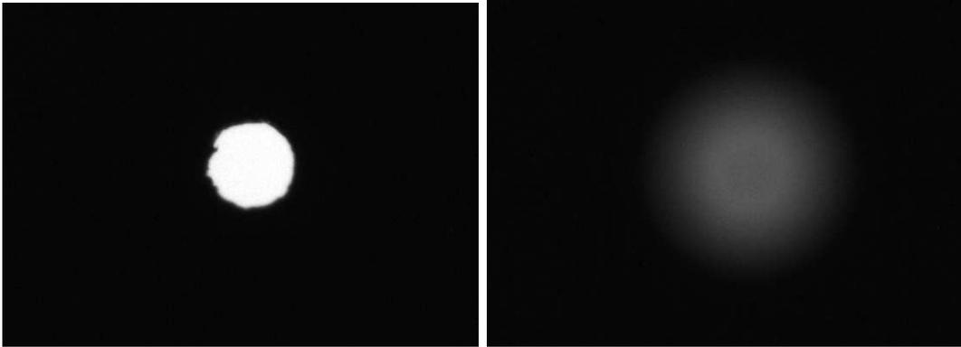
Figure 5.6 Actual focused and defocused pinhole images taken by the camera unit. The defocused image is 7.7 mm away from the focused image plane.
