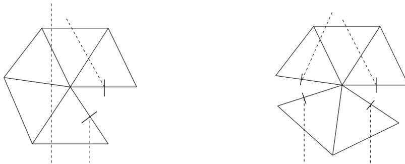
Figure 6.1: The paths of two initially parallel geodesics on a triangulated 2-d manifold, enclosing a vertex. As shown, representation is not unique, however, the total rotation of the two geodesics with respect to their initial paths always equals the deficiency of the enclosed bone.
