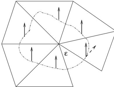
Figure 2.5: A vector parallel transported around a loop enclosing a bone comes back to its initial position rotated by an angle equal to the deficiency of that bone.
