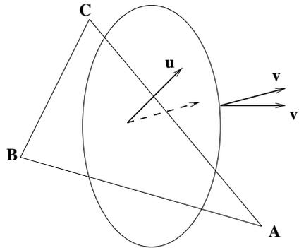
Figure 6.6: Vector  $\vec{v}$  is parallel transported around a loop enclosing Triangular bone  $ABC$ .
