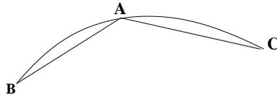
Figure 4.4: An arc segment is approximated using two line segments
