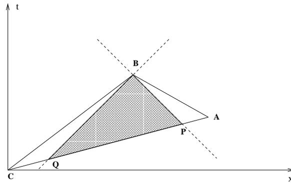
Figure 3.4: Triangle  $\triangle CBA$  is a SSS triangle and is broken into two NSS triangles,  $\triangle PAB$  and  $\triangle CBQ$ , and a NNS triangle,  $\triangle BPQ$  via the null cone of vertex B, here drawn with dashed lines.
