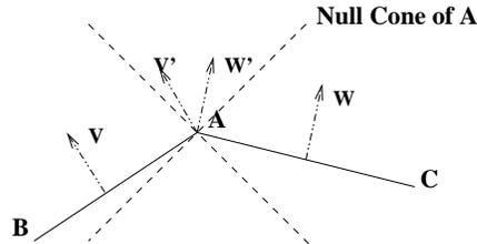
Figure 4.6: Vector  $\vec{V}$  is orthogonal to edge BA and vector  $\vec{W}$  is orthogonal to edge AC. One may define a normal at vertex A by taking a weighted average of them and measure the lapse of time using this normal. There is however no guarantee that this “Local” solution results into the same lapse of time for every vertex.
