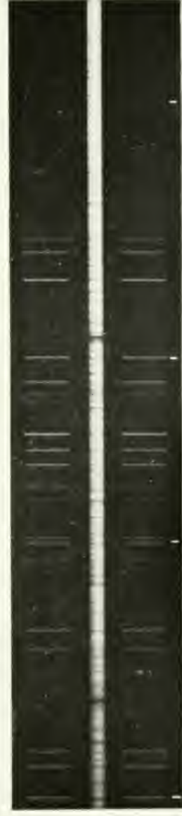
(a) (above) : The Hartmann focus test at settings 23.0, 24.0, 23.5 (b) (below) : The spectrum of HD 198726
