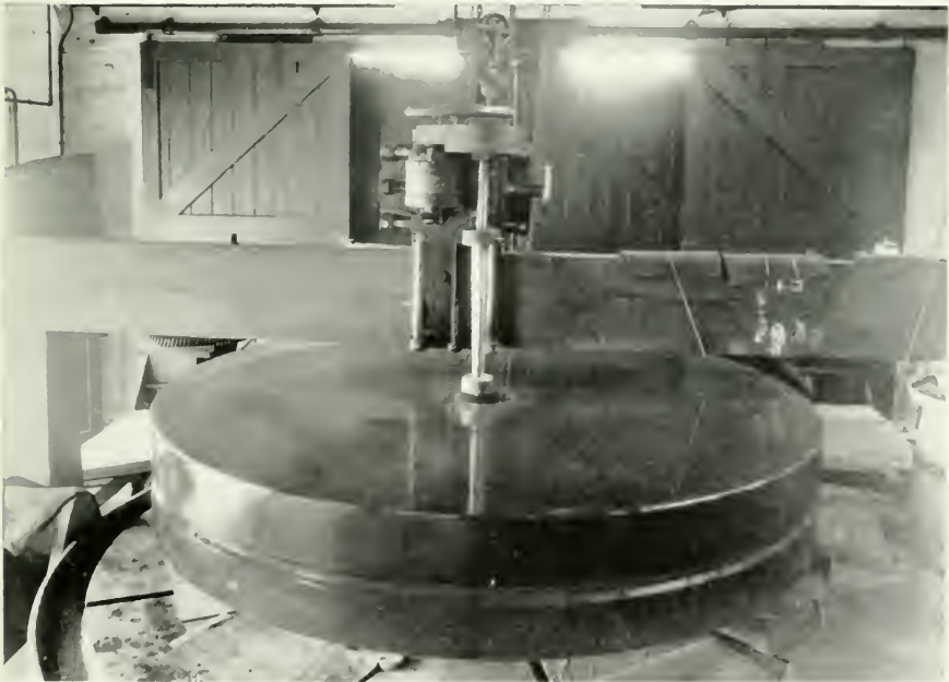
(above): The disk on its arrival in England (below): Grinding the central hole
