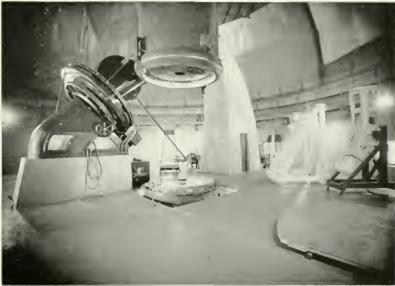
The hoist for removing the mirror for silvering
